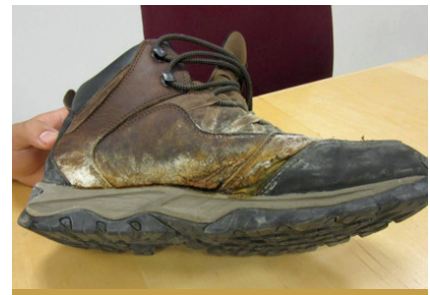
Leather work boot damaged during clean-up of sodium hypochlorite release.
