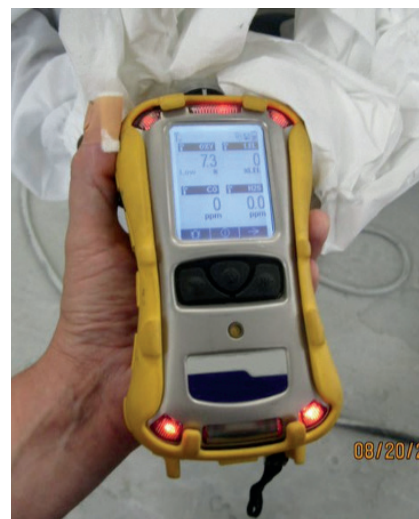
MultiRAE oxygen measurement in the respirator hood following the accident.
